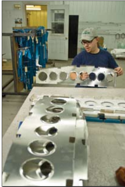
A Dream Aircraft employee prepares Tundra ribs for assembly into a quickbuild wing. Few items on the Tundra airframe are made outside of D&G.
