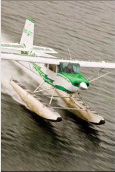
The 2300 straight floats that this Tundra has been tested on are undersized for the airframe, but there's more than enough hull available for a sexy one-float takeoff with three big guys aboard.
