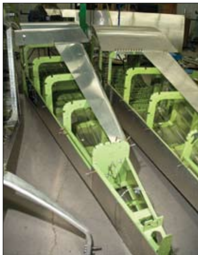
These quickbuild fuselages are being shipped with full interior chromating before being crated. Dream Aircraft takes pride in fulfilling specific customer needs when requested.
