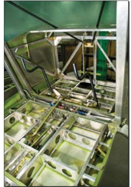
There’s a lot already done when you order the quickbuild option, including fuselage control cable runs and fuel system plumbing.
