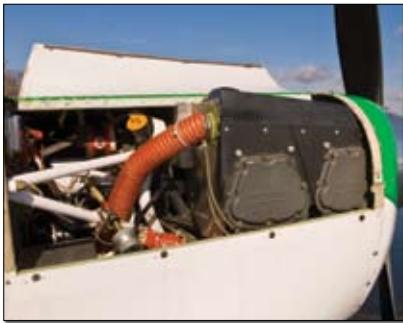
The 200-horsepower Lycoming IO-360 and constant-speed prop do a good job of overcoming the drag of the floats and rigging.
